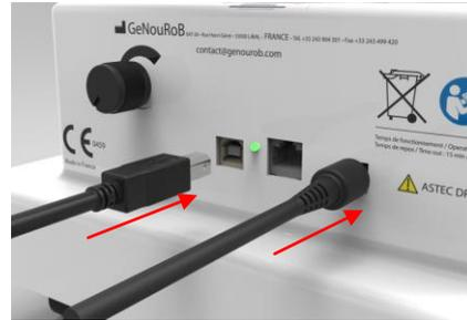
Connect the power supply bloc to the sector (**tension 100- 240 V ~ 2 A 50/60 Hz**).
