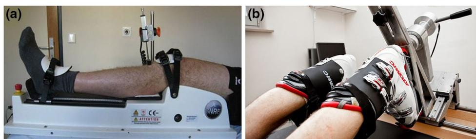
**Fig. 1** Anterior and rotational knee laxity measurement devices. **a** The GNRB<sup>®</sup>. The ankle and patella of the tested leg are fixed, and a motorised platform applies the anterior force behind the shank. The sensor placed on the tibial tuberosity measures the anterior displacement.
